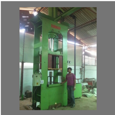
Deep Draw Hydraulic Press For Fire Extinguisher Shell
