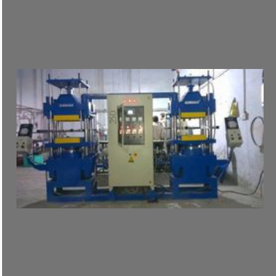
Hydraulic Press for Disc Brake Pad
