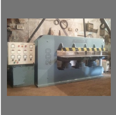
Rubber Conveyor Belt Jointing / Repairing Hydraulic Press
